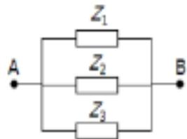
$$\frac{1}{\underline{Z}_{AB}} = \frac{1}{\underline{Z}_1} + \frac{1}{\underline{Z}_2} + \frac{1}{\underline{Z}_3} \Rightarrow$$
