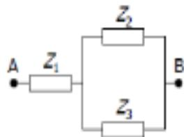
$$\underline{Z}_{AB} = \underline{Z}_1 + \frac{\underline{Z}_2 \underline{Z}_3}{\underline{Z}_2 + \underline{Z}_3}$$
