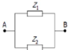
$$\frac{1}{\underline{Z}_{AB}} = \frac{1}{\underline{Z}_1} + \frac{1}{\underline{Z}_2} \Rightarrow \underline{Z}_{AB} = \frac{\underline{Z}_1 \underline{Z}_2}{\underline{Z}_1 + \underline{Z}_2}$$
